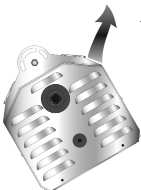
Figure 2.9 • Hot Flue Discharge
