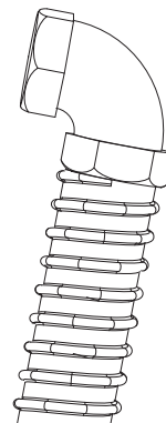
Figure 78: Liquidtight 3/4 Inch Elbow Connector Attached to Flexible Conduit.
