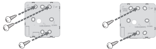
Figure 70: Location of the Controller Installation Plate Screws When Using a Handy Box.
