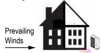
Figure 39: Leeward Side of the Building.
