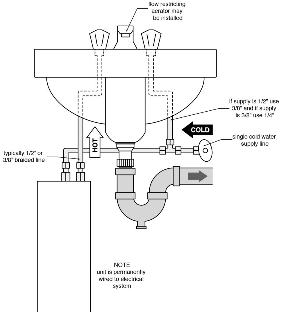
**4.** Open the hot water faucet and run water for minimum 60 seconds and until the flow is continuous and free of air pockets. Close the faucet and install the aerator (if supplied).
