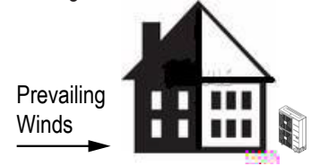
Figure 52: Leeward Side of the Building.
