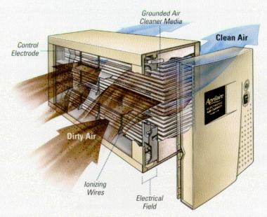
breakthrough technology that delivers recordsetting performance. Using air cleaning media instead of plates to trap particles provides several benefits. Unlike plate-type electronic air cleaners that lose efficiency over time, the Aprilaire Electronic
