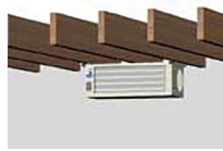
Horizontal air delivery; perpendicular to joists
