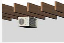
Vertical air delivery; recessed between joists
