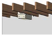
Horizontal air delivery; parallel to joists
