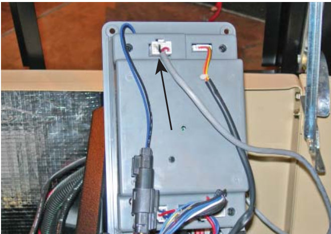
Figure 5B — Plug Wire Harness into 8-pin Header
