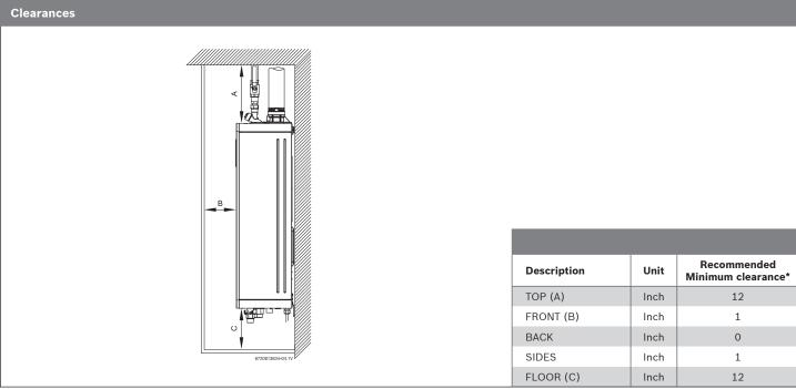
$<sup>^{\</sup>star}$  For servicing access, a 2ft clearance is recommended to the front cover.
