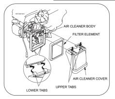
To service the air cleaner remove the air cleaner cover (1) by releasing two top catches (2) and tilting away from body until lower tabs release. Remove cartridge (3) and clean by tapping gently on a flat surface. If very dirty or damaged replace.
