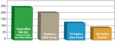
Data based on published manufacturer ratings for high-output models. Heat Input: Indirect 140,000 BTUH; Tankless 199,000 BTUH; Gas 70,000 BTUH; Electric 5500W
