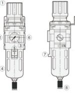
ADJUSTMENT KNOB To increase pressure , lift up on the knob and turn clockwise
