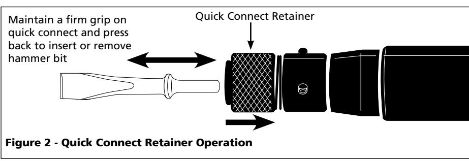
Figure 2 - Quick Connect Retainer Operation
