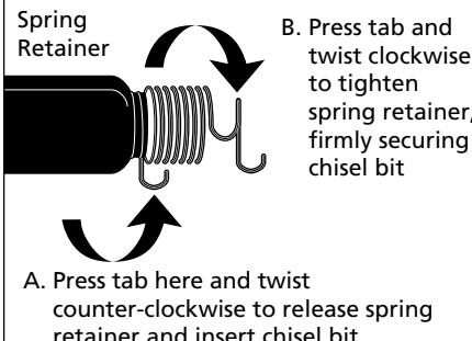
Figure 1 - Spring Retainer
