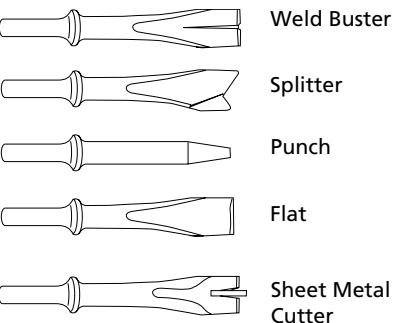
Figure 4 - Hammer Bits
