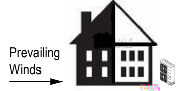
Figure 31: Leeward Side of the Building.
