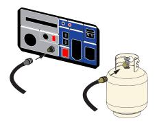
**Step 1:** Connect the included propane valve to the generator and to the propane tank. Open valve on propane tank.
