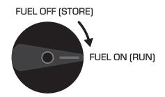
**Step 2:** Turn fuel switch clockwise to ON.
