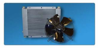
Splitbar Aluminum Radiator - this radiator serves two primary functions; one half of the radiator cools the oil to the pump. making it 100% duty cycle and the other function is to cool the (hot) outlet air to 10° from ambient temperature. This feature removes aproximately 50% of the humidity/water from the compressed air.
