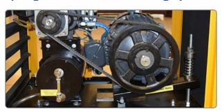
On 20HP units and below, we have a spring-loaded belt-tensioning device. This device keeps accurate belt tension on the compressor belts, which prevents excessive wear, reducing maintenance and downtime.
