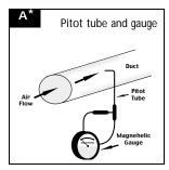
A The duct's airflow velocity is measured with a magnehelic gauge and a pitot tube. See "Pitot Tube Balancing Procedure" next page.
