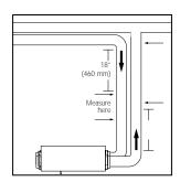
To avoid airflow turbulence and incorrect readings, the airflow velocity should be measured on steel ducting a minimum of 18" (457 mm) from the unit or elbow and before any transition.
