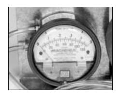
2 Before taking the reading, make sure that the magnehelic gauge is level and at 0. Refer to the flow measuring station's chart to determine your unit's airflow velocity.
