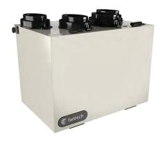
A great mid-range heat recovery ventilator, the VHR100R ES is ideal for high-rise apartment applications, condominiums, single and multi-family homes. With its compact top port design featuring 5 inch oval collars and the included EZ-MountTM wall bracket, the VHR100R ES can be installed in spaces as small as 24 inches, such as a closet or maintenance room.
