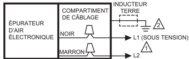
1 BLOC D'ALIMENTATION. PLACEZ SI NÉCESSAIRE UN DISPOSITIF DE COUPURE ET UNE PROTECTION CONTRE LES SURCHARGES.
