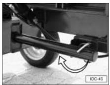
Secure the log lift tray in the UP and LOCKED position using the safety pin and hairpin clip.
