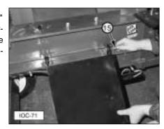
**17**. Raise the log lift arm. Align the attachment plate and lift cylinder rod.
