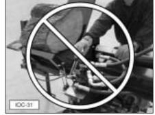
Make sure both ends of the log you are splitting are cut as square as possible. This will prevent the log from sliding out of position while under pressure. All logs should be 24 inches long or shorter.
