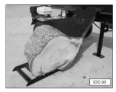
5. Raise the log lift using lever (3), slightly past horizontal.
