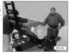
7. Fully raise the log lift using lever (3) and center the log on the rail assembly.
