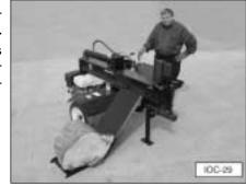
If a second person is assisting the operator, extreme caution must be observed. It is the operator's responsibility to keep the second person from being injured while the log splitter is being operated. The operator must not initiate movement of the pusher plate, log lifter, or 4-way wedge unless all hands, feet, or other body parts are clear. It is best for safe operation if the second person loads logs onto the lift, but only the operator positions the log for splitting.
