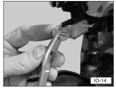
12. Attach the valve handle to the valve spool using a 1/4 x 1 inch long clevis pin. Secure the clevis pin with a cotter pin (bend the ends of the cotter pin to make it secure). Attach the knob to the valve handle, if necessary.
