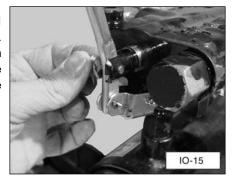
13. Attach the high-pressure hose from the filter assembly to the fitting on the side of the valve. Securely tighten the hose fitting.
