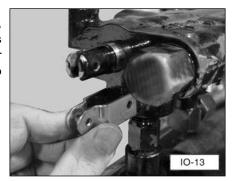
11. Install the valve handle onto the valve link using a 1/4 x 3/4 inch long clevis pin. Secure the clevis pin with a cotter pin (bend the ends of the cotter pin to make it secure).
