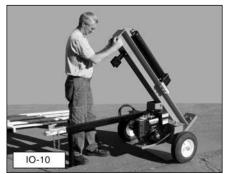
**8.** Link the ends of safety chains together with the safety quick-link and tighten the link's locknut securely with a wrench.
