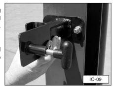
7. Block the wheels to prevent the base unit from moving. Carefully lower the rail assembly to a horizontal position. Securely tighten the nuts holding the base unit to the rail assembly (Step 5) and the nuts holding the rail rest assembly (Step 6).
