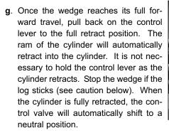
h. DO NOT load another log or remove split pieces until the wedge has completely stopped and the control handle automatically returns to the neutral position.
