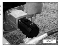
15. Remove the oil filter from the plastic cover and apply a thin coat of oil to the rubber seal. Screw the filter onto the filter head, located near the hydraulic tank. Once the filter makes contact with the filter head, turn it an additional 3/4 turn. Hand-tighten only.
