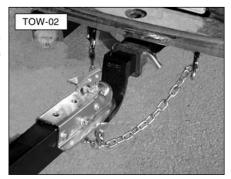
Raise the front leg to the towing position by pulling the spring pin. If not already secure, make sure the hitch coupler is properly and securely attached to the tow hall
