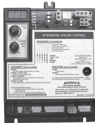
Figure 17: Integrated Boiler Control
