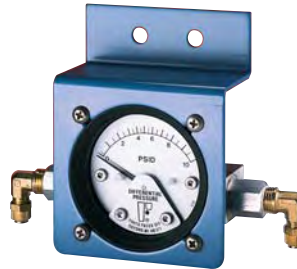
KBDPI-25 Differential Pressure Gauge Temp: 200°F (88°C) Pressure: 250 PSIG (17 bar) (Kit includes 1/8" and 1/4" NPT brass fittings, flex ble nylon tubing and mounting bracket)
