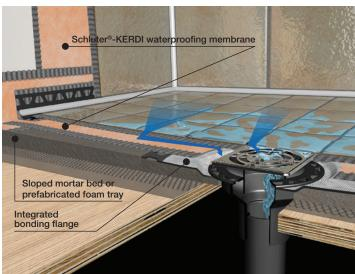
The traditional method for installing tiled showers is both time and labor intensive and requires many steps to ensure success.
