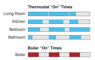
With synchronization, the cycle start times are coordinated between zones to allow for longer on & off times. Reducing equipment short cycling prolongs the boiler life & improves system efficiency.
