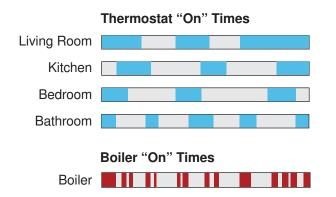
Without synchronization, the boiler is at the mercy of each zone. Non-communicating thermostats short cycle the boiler to achieve independent targets rather than systemwide goals. Boiler operation is inefficient & unreliable.
