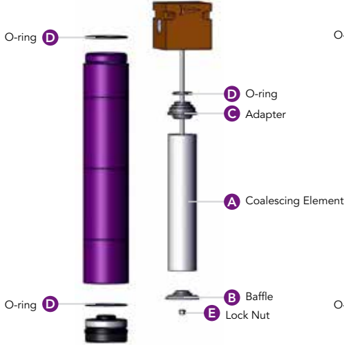
Figure 4 : Oil Coalescing Filter
