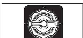
2. For propane, rotate the fuel selector switch to **LPG** and open the propane cylinder valve.
